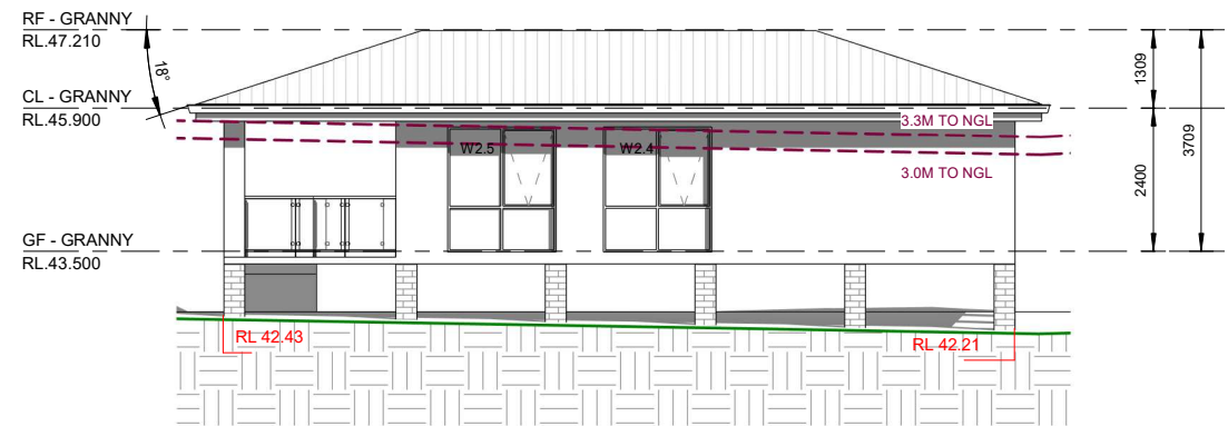
4 SOUTH EAST ELEVATION - GRANNY FLAT 1 : 100
