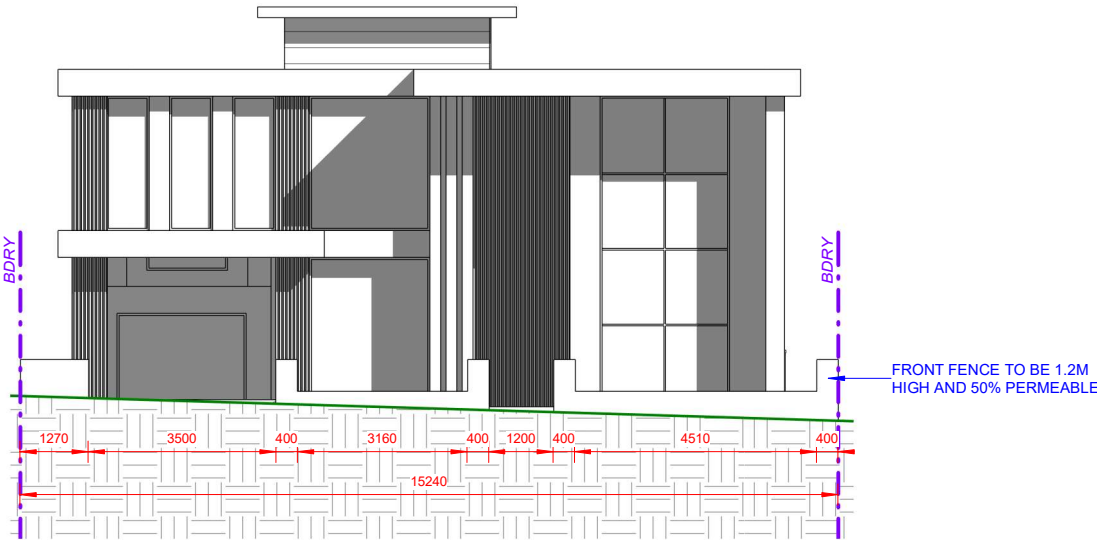
2 FRONT FENCE ELEVATION 1 : 100
